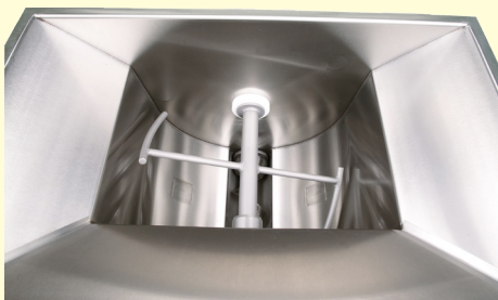
PADDLE SHOWN INSTALLED IN HOPPER
