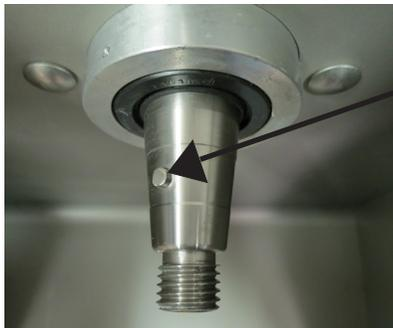
There is an alignment pin on the lower shaft. And a mating alignment groove in the hub of the lower wheel. Align the two as the wheel is being installed on the tapered shaft.
