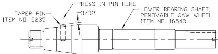
If there is no groove (keyway) in the bore of the lower wheel, discard the taper pin and use the shaft without the pin.
