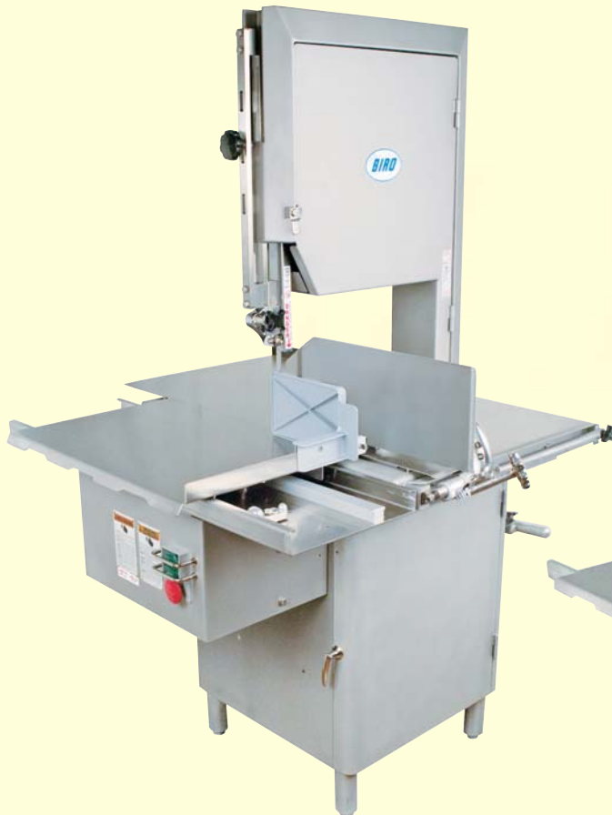
Md. 44SSLP custom Low Profile, high speed, portion control Power Cutter, equipped with a standard meat thickness gauge. See reverse side to view the optional micro meter thickness gauge fence.
